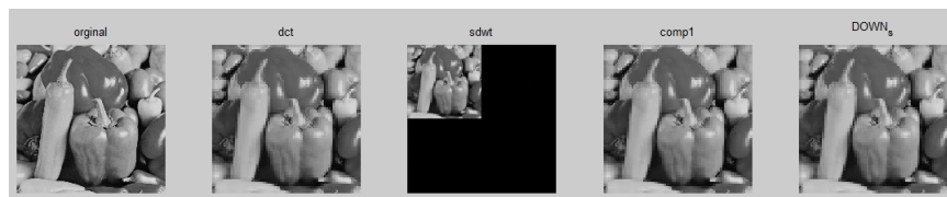
Figure 6: Comparison of the proposed image compression methods.
