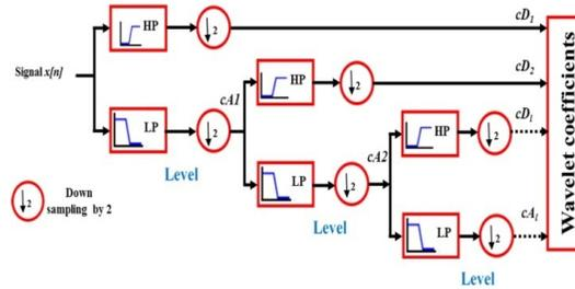
**Figure 2:** Signal decomposition using discrete wavelet transform
